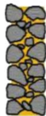
Traditionally built wall
