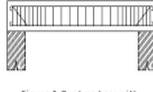
Figure 3 - Bent-up bars with Vertical Stirrups
