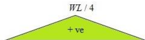
(c) Bending Moment Diagram
