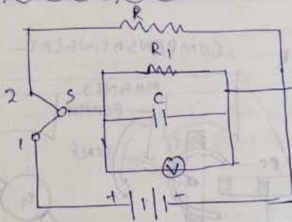
(i) In the circuit, C is capacitor of known capacitance. V is voltmeter,  $R_1$  = total leakage resistance, and  $R$  = resistance to be measured.
