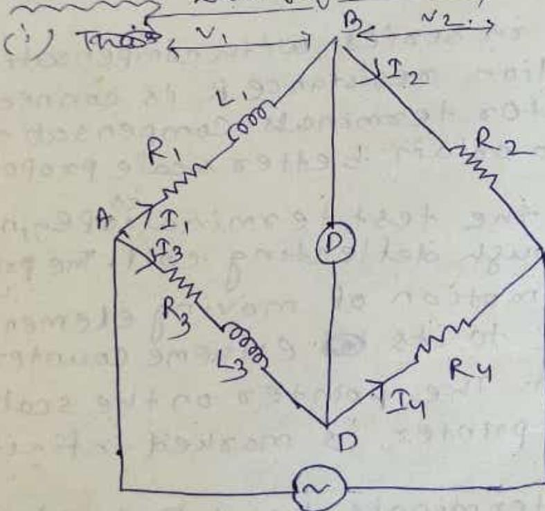
(i) It is used to measure the medium resistance.
