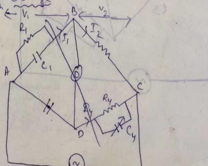
It is used to measure capacitance.
