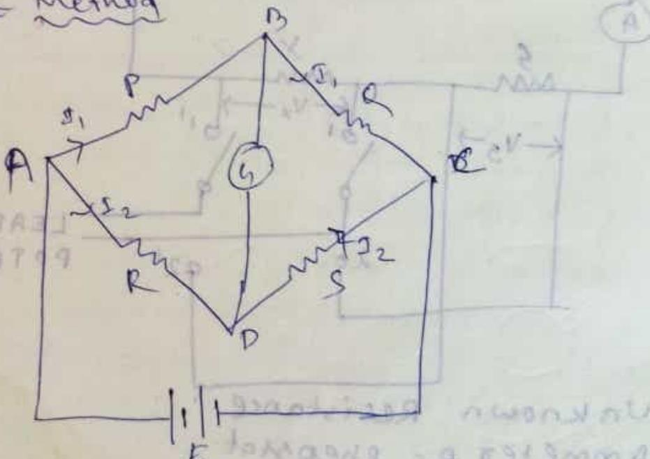
(i) It is used for measurement of medium resistance. It has four resistive arms P, Q, R and S and one galvanometer.
