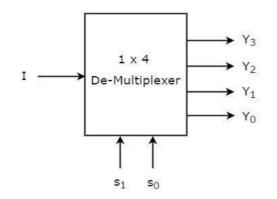
The single input 'I' will be connected to one of the four outputs,  $Y_3$  to  $Y_0$  based on the values of selection lines  $s_1 \& s0$ .
