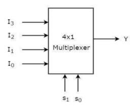
One of these 4 inputs will be connected to the output based on the combination of inputs present at these two selection lines.
