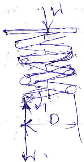
① Torsional shear of the helical spring
