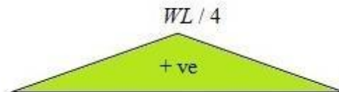
(c) Bending Moment Diagram
