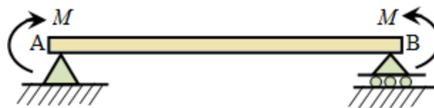
(a) Simple supported beam with end coupling
